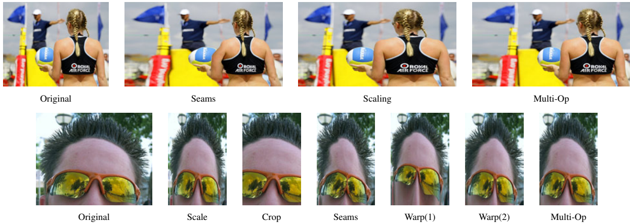
Figure 12: Comparison of retargeting results (expansion and reduction) using various image retargeting methods. These examples illustrate cases where using optimized multi-operator retargeting combining seam carving, cropping and scaling achieves better results. Seams is using seam carving from [Rubinstein et al. 2008], Warp(1) and Warp(2) are non-homogeneous scaling from [Wang et al. 2008] and [Wolf et al. 2007] respectively.
