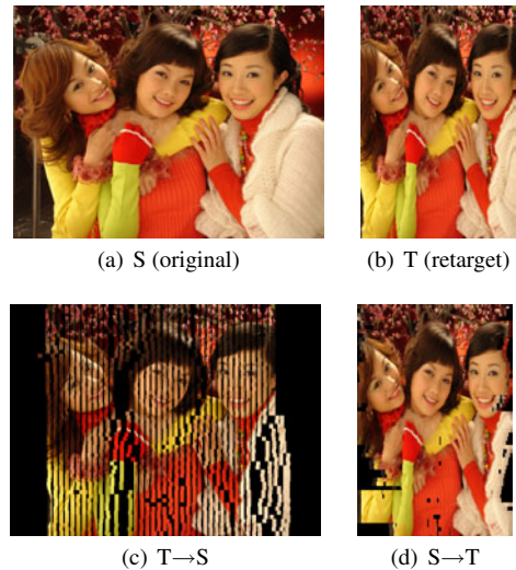
Figure 8: BDW uses two alignments of the source image to the retargeted image and vice versa. The distance would be the maximal matching cost of elements in the two. Note how the alignment reveals that the retargeting used a combination of cropping (gaps on the sides of the alignment), scaling (uniform spacing between patches in the middle) and seam carving (large gaps in the middle).
