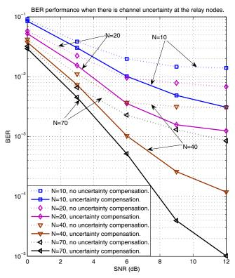
Figure 3: The BER comparison when the channel uncertainty compensation scheme in (22) is used vs. the relay scheme in (7) assuming  $10\log\sigma_{\Delta_s}^2/\sigma_s^2 = 10\log\sigma_{\Delta_t}^2/\sigma_s^2 = -10$  dB uncertainty at the relay sensor nodes.
