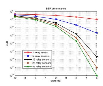
Figure 2: The BER performance of the proposed scheme(7) when the relay sensors are assumed to have more noise power than the destination sensor. The relay sensors are placed such that they have the same distance from the source and destination sensors.
