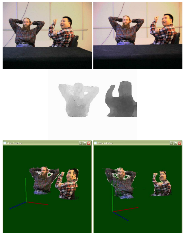
Figure 6: Typical results from our real-time online stereo system. The first row shows the two input images, while the second row shows the disparity map and the reconstructed 3D point cloud from different perspectives. Some holes in the 3D views are caused by the rendering. We simply render fix-size (in screen space) points using the GL_POINT primitive.
