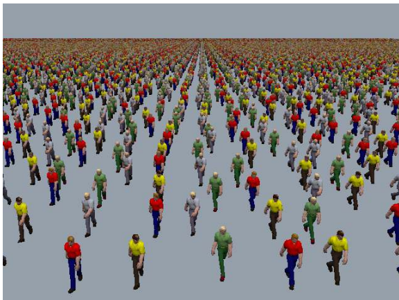
replicated poser models, 90000 objects, 575 million triangles, rendering time 294 msec (splat size 2 \times 2 )
