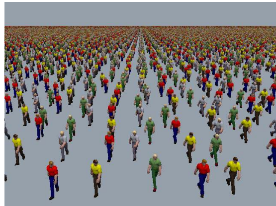
(d) replicated poser models, 90000 objects, 575 million triangles, rendering time 294 msec (splat size 2×2)
