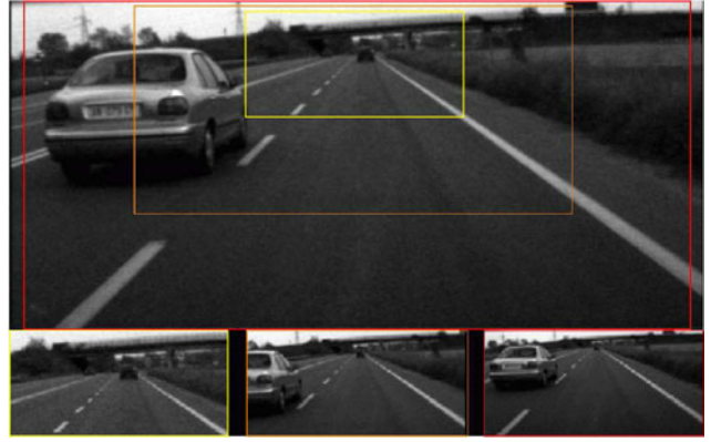
Fig. 3. Interest areas for the detection of: far (left), medium distances (center), close (right) vehicles.
