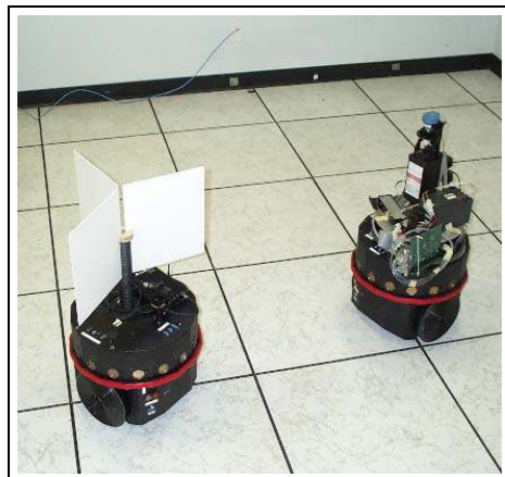
Figure 1: Two robots, one equipped with laser range finder (right) and the other with a target (left), employing cooperative localization.
