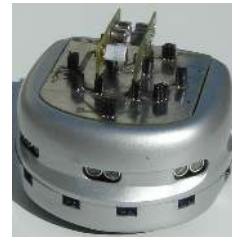
Fig. 3. Khepera III and kheNose with sensing modules
