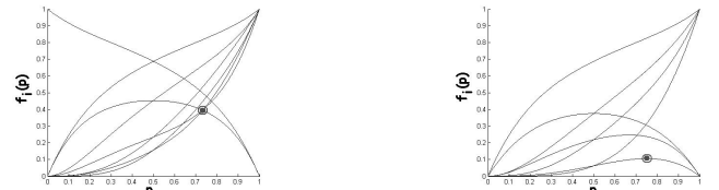
Fig. 5. An illustration of two possible maximin points. On the left, the point is created by the intersection of two curves, and on the right it is the local maxima of the lowest curve.
