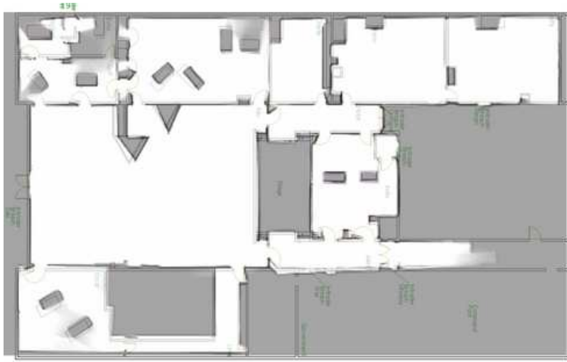
Fig. 8. Combined map for all four robots using the multi-robot SLAM algorithm. One pair of robots starts from the right-top room, the other from the right-bottom corridor. The map is shown overlaid on the ‘ground-truth’ blueprint.
