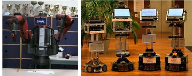
Fig. 1: Baxter manipulator and CoBot mobile service robots coordinated with the proposed approach.
