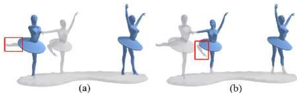
Figure 19: Limitation to the use of intrinsic distances (a 3D case). Our method returns erroneous symmetry regions in the first two scales (a-b). The input model is the same as the one in Figure 1 except that the last dancer now has both feet planted into the base, creating a topological inconsistency among the three dancers. Symmetry detected for the remaining scales are the same as Figure 1.
