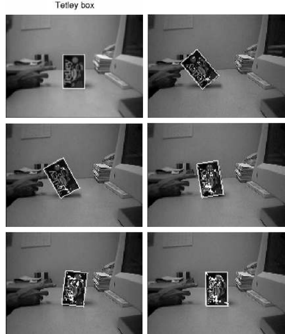
Figure 5: Top left image: segment of the image selected by the user to define the “tetley box” model. Remaining images: the light points inside the rectangles represent the interest points used for the best similarity match.
