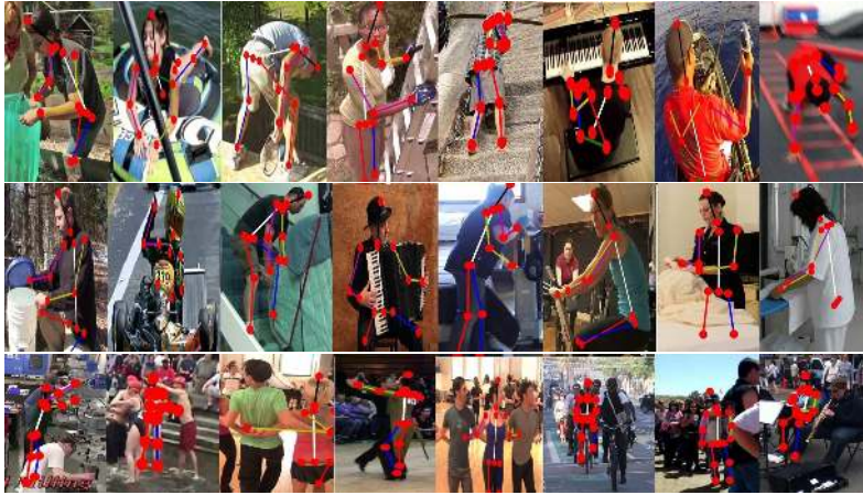
Fig. 1. State-of-the-art pose estimation networks face difficulties in diverse activities and complex scenes, which can be organized into three challenges: (top row) large scale varieties of body keypoints in the scenes, (middle row) occluded body parts or keypoints, (bottom row) ambiguities in matching multiple adjacent keypoints in crowded scenes.
