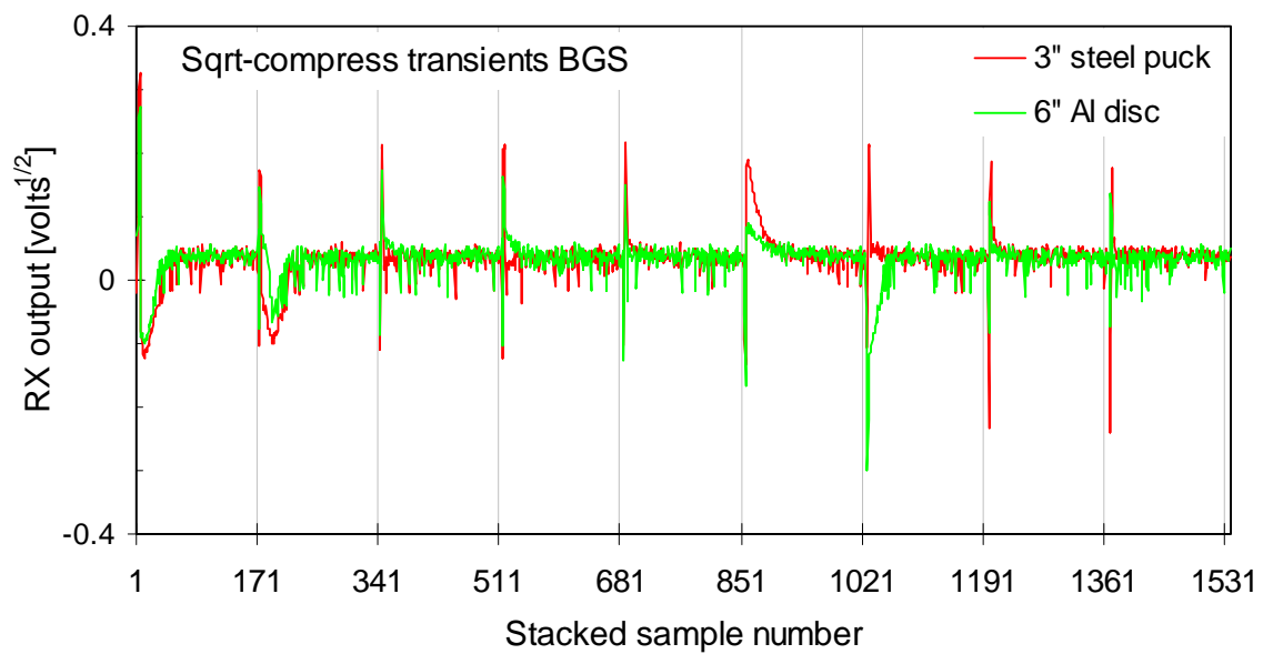
Figure 32. Stacked EMI transients for the entire 9-RX array. The signals in the bottom panel are background-subtracted. The transients are shown sequentially from left as: RX8, RX1, RX3, RX6, RX4, RX5 (central loop), RX2, RX0, RX7.
