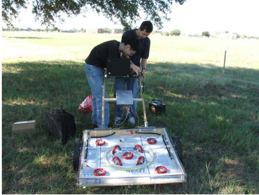
Figure 26. Complete one-man-portable EMI system prototype.
