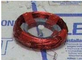
Figure 6. Photograph of a receive loop antenna.
