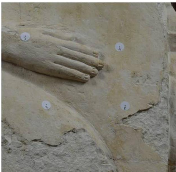
Figure 8. Some circular sticky stamps used to materialize TX and RX points.
