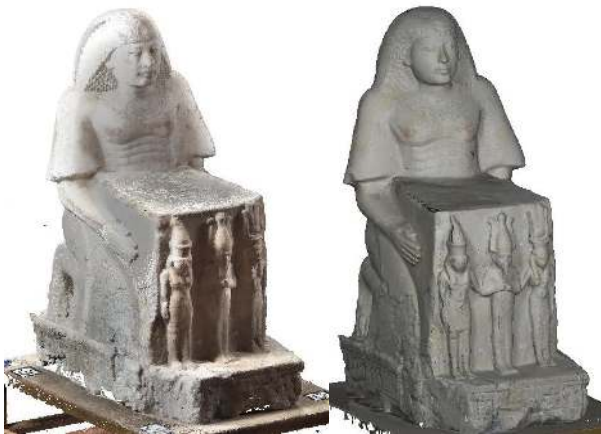
Figure 3. Laser Freestyle point cloud and textured mesh.
