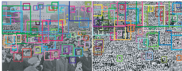
Figure 2: Results of Head Detection: Image on the left is one of the few images where head detection gives reasonable results. False negatives and positives are still evident in both images.
