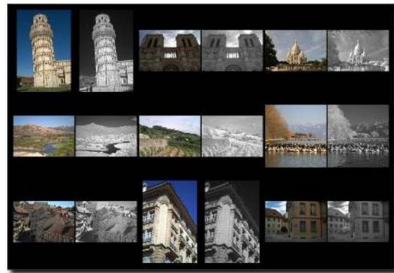
Figure 1: Examples from our database of RGB-NIR images. Notice that the NIR band exhibits noticeable differences at the scene level: sky and water are dark, foliage is bright, and details are more clearly resolvable in haze.
