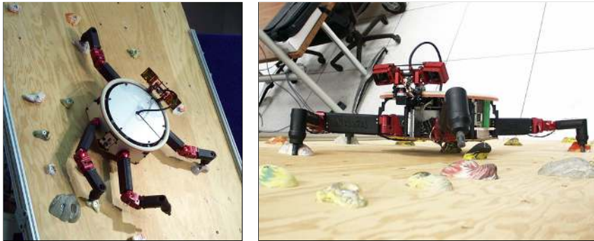
Fig. 1. LEMUR I Ib, a multi-use robot capable of free-climbing (Mechanical and Robotic Technologies Group, Jet Propulsion Laboratory) [9].
