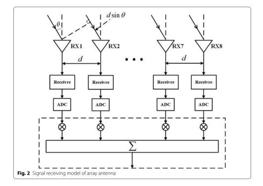
Based on the above equation, the phase change of the *i*-th receiving antenna is
