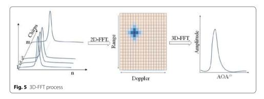
different angles has its own unique law of phase change. As a result, it is possible to separate targets with different frequencies by performing Fourier analysis on multiple echo signals. We propose a 3D-FFT estimation approach and construct RAM to separate the multiple targets. The detailed operation procedure of 3D-FFT is shown as in Fig. 5.
