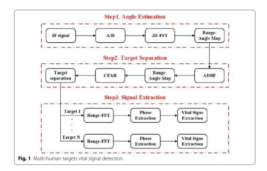
information. Then, the interference between multiple targets is weakened and the target signal is enhanced by ADBF technology. Afterward, multiple human target signals are separated on RAM by CFAR method. Finally, the separated individuals are detected for vital signals.
