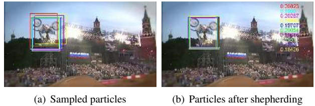
Figure 2. The multi-task correlation filter can be used to shepherd the sampled particles toward the modes of the target state distribution. The numbers in (b) are the scores of correlation filter for the particles. Different colored boxes indicate the respective locations and scores.
