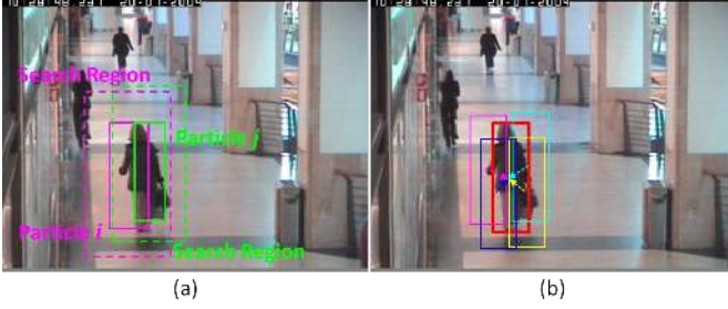
Figure 3. The MCPF can cover object state space well with a few particles. Each particle corresponds to an image region enclosed by a bounding box. (a) The MCPF can cover object state space well by using few particles with the search region where each particle covers the state subspace corresponding to all shifted region of the target object. (b) The MCPF can shepherd the sampled particles toward the modes of the target state distribution, which correspond to the target locations in the image.
