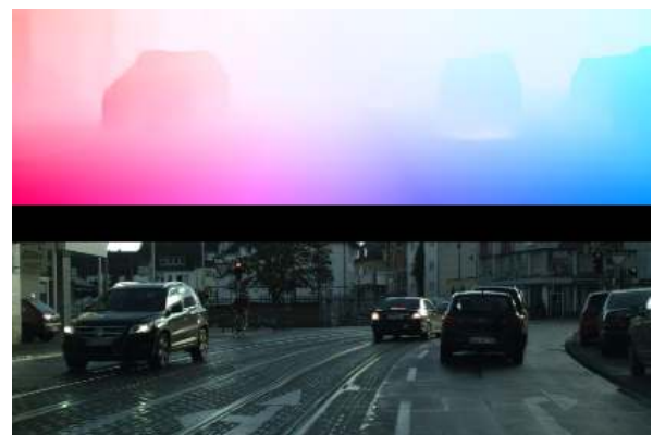
Fig. 1: The optical flow feature as a better cue for learning control signals We proposed to generate the optical flow feature (upper) that highlights movement across frames from a color dash camera frame (lower). Such a feature is a powerful cue in learning self-driving car controls.
