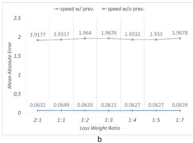
Fig. 11: Experiment results of multi-task network with/without using the speed ratio. (a) Yaw rate prediction of multi-task CNN with different loss weight ratios. (b) Speed prediction of multi-task CNN with different loss weight ratios.
