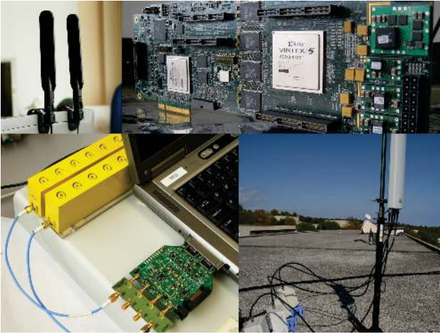
Figure 4. Hardware modules of the OpenAirInterface: CBMIMO1 card (bottom left) and Express MIMO card (top right), UE antennas (top left) and BS antennas with power amplifiers (bottom right)
