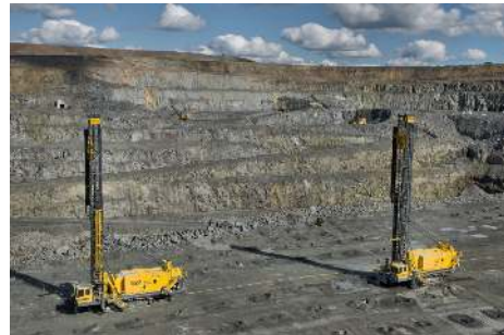
Fig. 1. Two Atlas Copco drilling machines (Pitviper-351) in the process of drilling targets in a bench.
