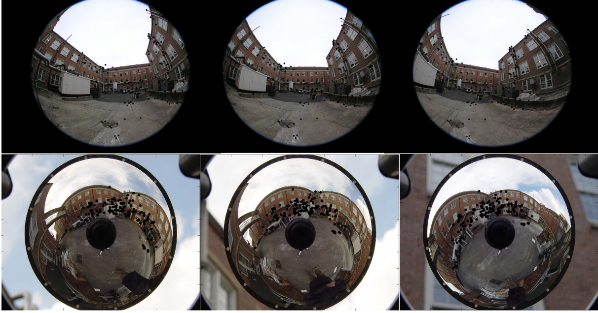
Figure 7. The triplet of images input to the system with features that were automatically matched overlaid. Top: Fish-eye images Bottom: Catadioptric images
