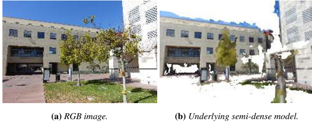
Figure 2: In this semi-dense reconstruction, the trees are only partially modeled and thus ray-casting will not work for automatic disambiguation of 2D annotations. This model was created using MVE [Fuhrmann et al. 2015] and contains 993,506 points; it corresponds to the sparse Campus2 dataset in Table 1.
