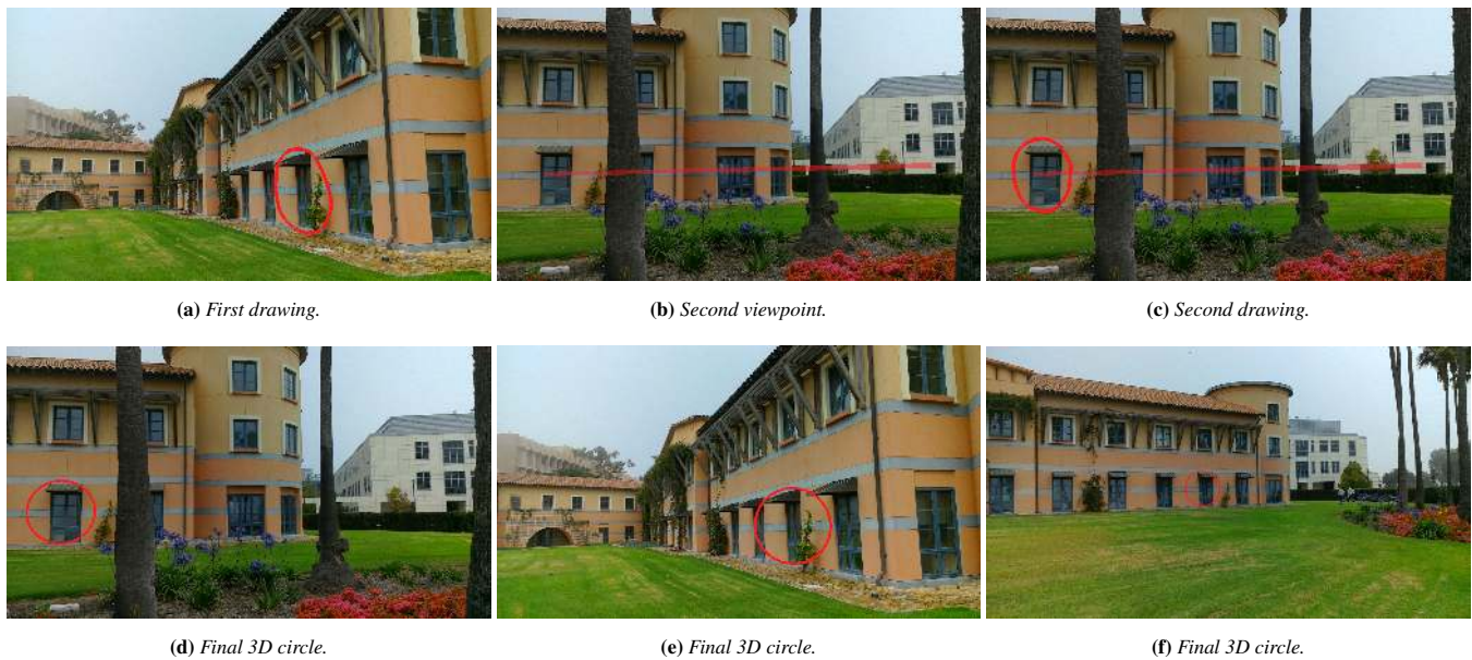
Figure 11: Screenshot of annotating in the Campus1 dataset. The user draws an annotation (a) and automatically sees a second viewpoint for disambiguation (b) with a semi-transparent line l of the same color as the annotation. A second drawing (c) determines the final 3D circle as seen from different viewpoints (d-f).
