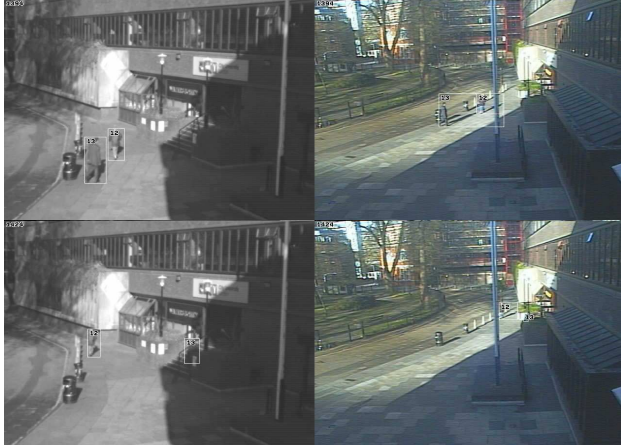
Figure 3: Example of handling dynamic occlusion. The top, and bottom images show two objects before and after a dynamic occlusion. The correct labels are still assigned after the occlusion.
