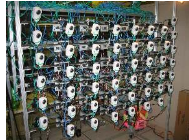
Fig. 1. Our self-reconfigurable camera array system with 48 cameras.
