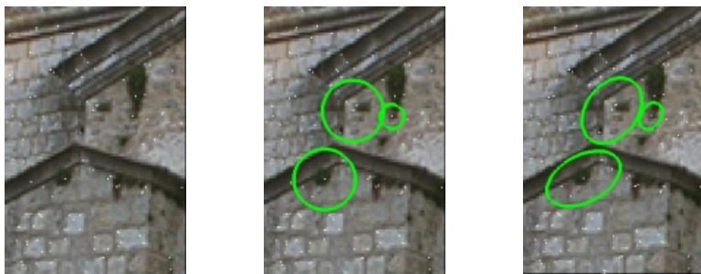
Fig. 3. Invariant neighbourhood process. Left: close-up of original image. Middle: three detected interested points, their associated scale indicated by the size of the circles. Right: the corresponding affine-adapted neighbourhoods.
