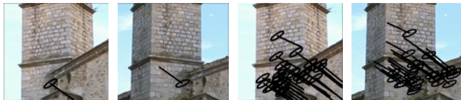
Fig. 9. A seed match (left) and the 25 new matches grown from it (right).
