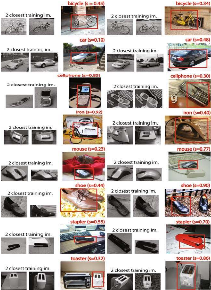
Fig. 8.15 Estimated pose for each object that was correctly classified by the algorithm. Each row shows two test examples (the colored images in column 3 and column 6) from the same object category. For each test image, we report the estimated location of the object (red bounding box) and the estimated view-synthesis parameter s . s gives an estimate of the pose as it describes the interpolating factor between the two closest model (canonical) views selected by the recognition algorithm. For visualization purposes we illustrate these model views by showing the corresponding training images (columns 1-2 and 4-5). Images belong to the dataset in [55].
