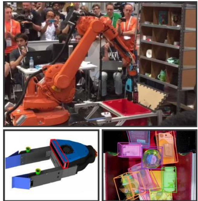
Fig. 1. Top: The MIT-Princeton robotic picking system. Bottom-left: The gripper mounted with an Intel RealSense camera (outlined in red). Bottom-right: Predicted 6D object poses from our vision system during the stow-task finals of the APC 2016. Each prediction is highlighted with a colored 3D bounding box.
