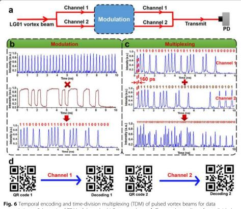
transmission. **a** Schematic of TDM of the pulsed  $LG_{01}$  vortex beam. **b** Temporal encoding of one divided pulsed vortex beam. **c** Multiplexing of two encoded pulsed vortex beams. **d** Measured data transmission results for two QR codes transfer using temporal encoding and TDM of pulsed vortex beams
