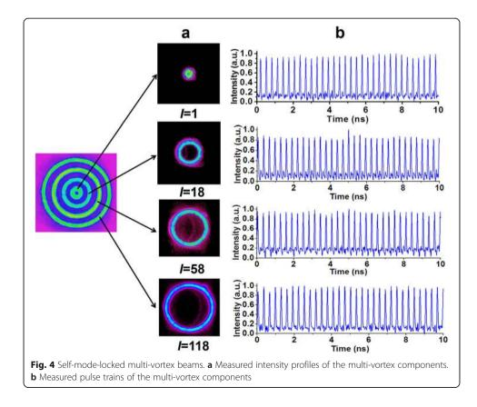
Remarkably, the obtained results show that the generated multi-vortex beams are naturally decomposable and coaxial. Moreover, the multi-vortex beams carry highrepetition picosecond pulses. Therefore, compared with traditional single-charge continuous wave (CW) vortex lasers, the developed multi-vortex laser increases two available spatial and temporal dimensions, which provides favorable potential to perform spatial and temporal encoding for data transmission.
