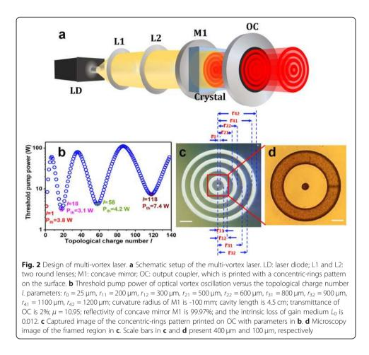
pattern can be completely described by the radius of the central circle  $r_0$ , the inside radius of the *i*-th ring  $r_{i1}$ , the outside radius of the *i*-th ring  $r_{i2}$ , and the number of the rings *n*.
