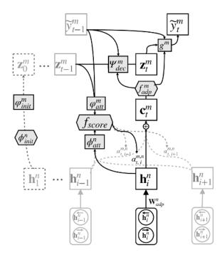
Figure 1: One step of the proposed multi-way. multilingual Neural Machine Translation model, for the n-th encoder and the m-th decoder at time step t. Shaded boxes are parametric functions and square boxes represent intermediate variables of the model. Initializer network is also illustrated as the left-most network with dashed boxes. Notice, all the shared components are drawn with diamond boxes. See Sec. 4 for details.
