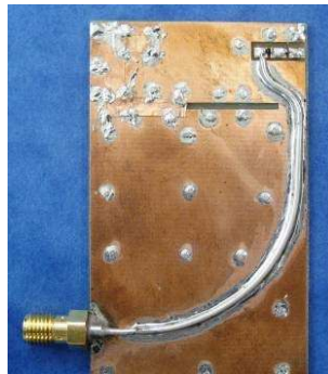
Figure 8. Transmission line arrangement in ground plane with a short-ended slot. As explained in Section 2, the advantage of slots with shorted ends is their situation in the ground plane. PCB design becomes more flexible as it exists a direct way for the transmission line for connecting the feeding port and the RF module [5].
