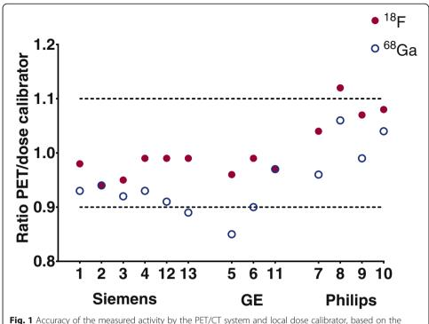
**Fig. 1** Accuracy of the measured activity by the PET/CT system and local dose calibrator, based on the average between the cylindrical and IQ phantom. Numbers correspond to Table 2
