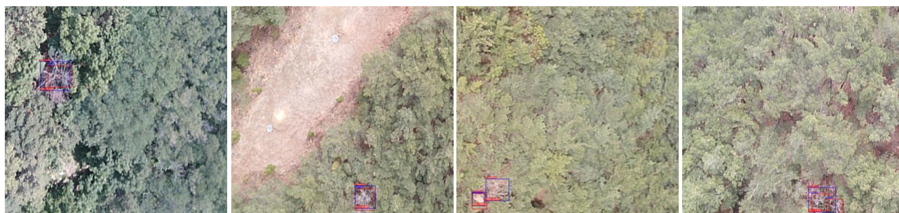
Fig. 7. Detection visualization of RGB images based on browning and dead trees. The blue box is the labeled ground true area, and the red box is the area predicted by the trained model.
