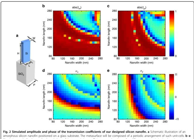
amorphous silicon nanofin positioned on a glass substrate. The metasurface will be composed of a periodic arrangement of such unit-cells. **D–e** Simulation results for the amplitude and phase of the transmission coefficients  $t_{xx}$  and  $t_{yy}$  shown for a 2D parameter optimization by using a rigorous coupled wave analysis method. The length and width of the nanofin are both swept in the range of 80–280 nm at an incident wavelength of 800 nm
