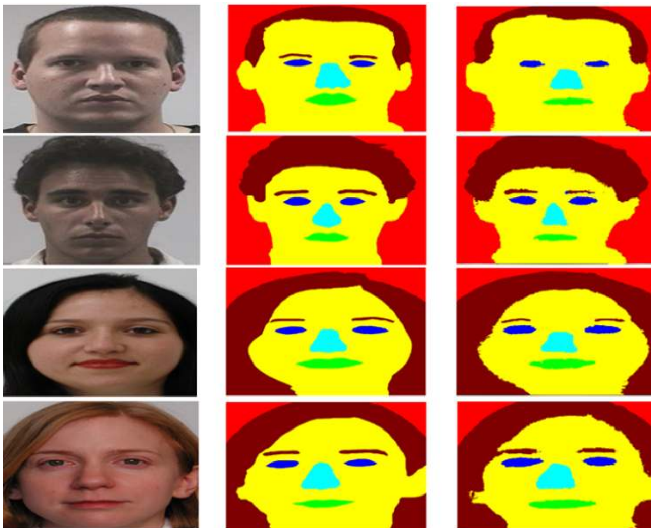
Figure 1. Images from the FASSEG V-4 database. First column shows original RGB images, second column shows ground truth images, and third column shows results obtained with the proposed MSS-CRF (better segmentation results).
