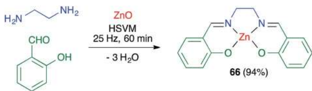
Scheme 46 Mechanochemical synthesis of a zinc–salen complex.
