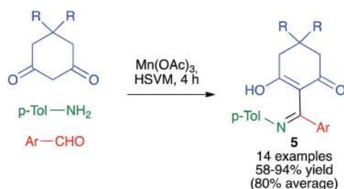
Scheme 6 A radical Mannich-like oxidative process under high-speed vibration milling.
