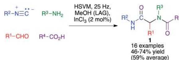
Scheme 1 The mechanochemical Ugi reaction.
