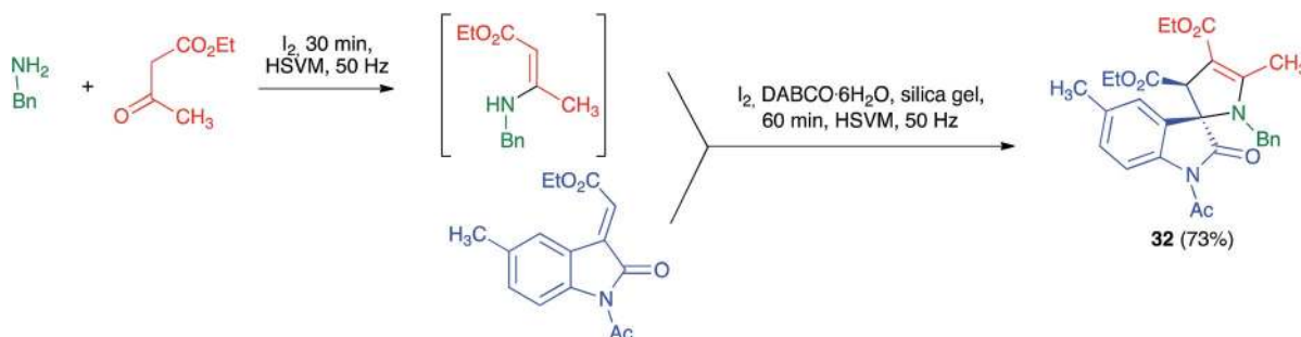
Scheme 21 Mechanochemical synthesis of 3,2'-pyrroline-spirooxindoles from in situ -generated \beta -enaminoesters.
