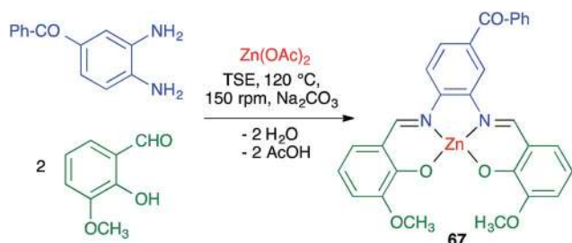
Scheme 47 Preparation of a salicylaldehyde imine complex under twin screw extrusion.
