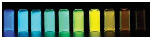
Fig. 3 Emission solvatochromism of compound 26b (recorded in cyclohexane, toluene, THF, EtOAc, acetone, \text{CH}_2\text{Cl}_2 , MeCN, i PrOH, EtOH, MeOH (from left to right); T = 293 \text{ K} ; c(\mathbf{26b}) = 10^{-4} \text{ M} ; \lambda_{\text{excit}} = 356 \text{ nm} , hand-held UV lamp). Reprinted with permission from J. Org. Chem. , 2014, 79 , 3296–3310. Copyright 2014 American Chemical Society.
