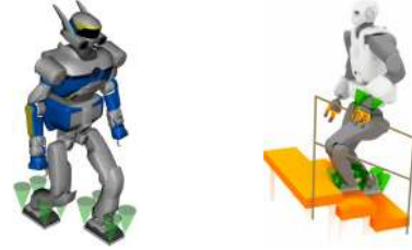
Fig. 1. Illustration of HRP-2 robot and TALOS robot making contacts with their environment. The green “ice-cream” cones are dispatched on the 4 vertices of the feet, symbolizing the friction cones with friction coefficient of value 0.3.
