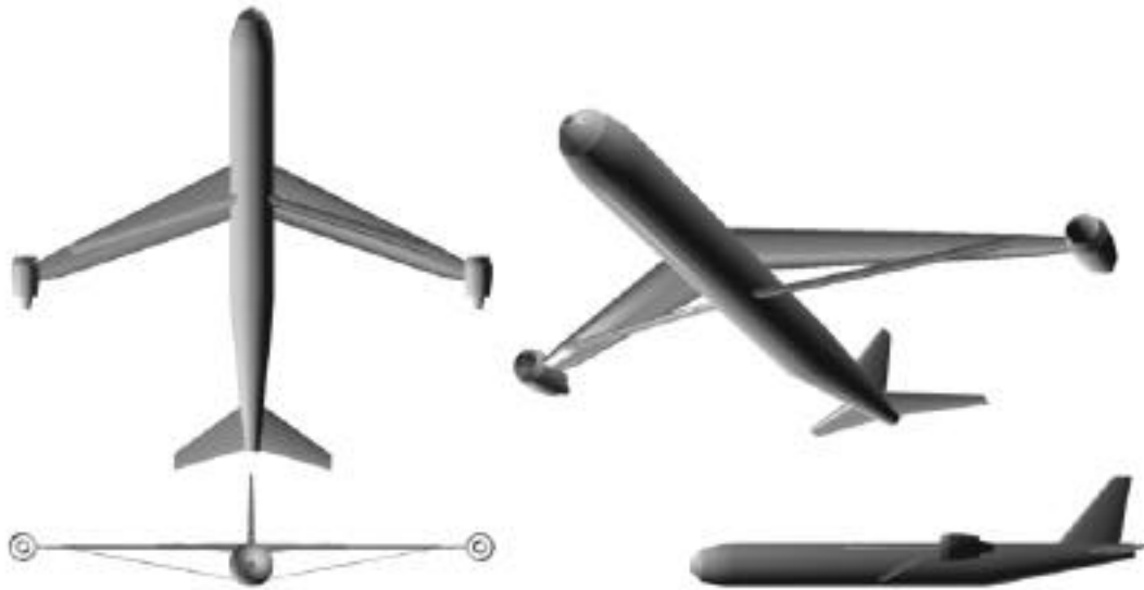
Figure 4-3: Optimum single-strut configuration with tip-mounted engines
