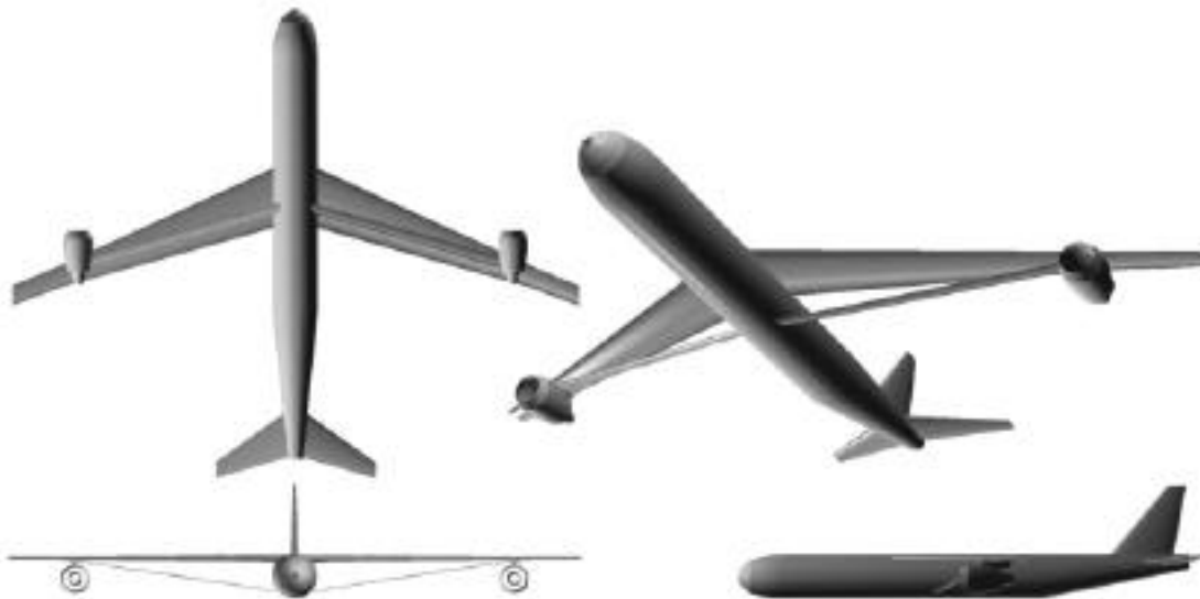
Figure 4-4: Optimum single-strut configuration with under-wing engines*
