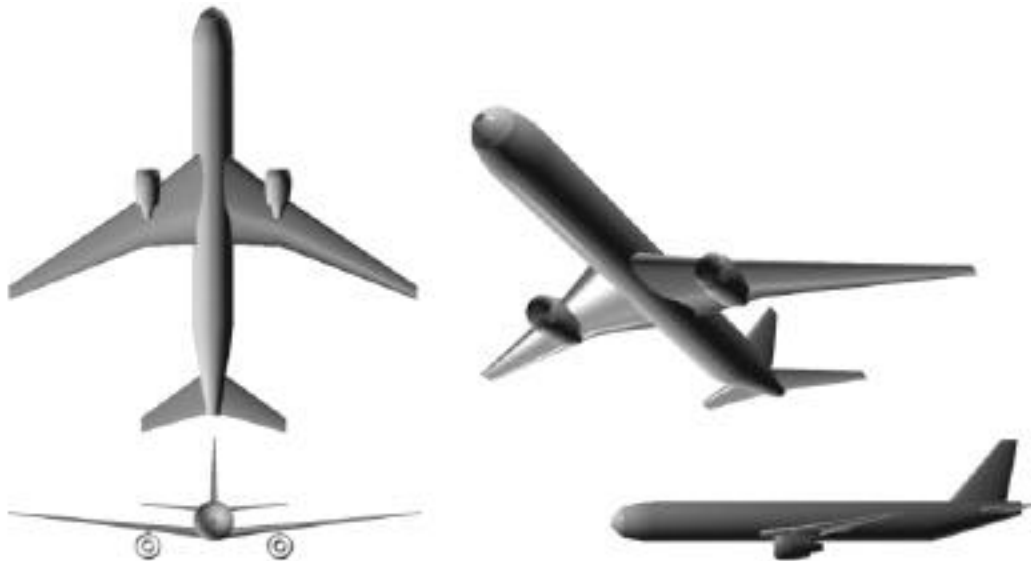
Figure 4-2: Advanced technology optimized cantilever configuration
