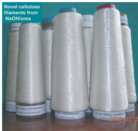
Figure 1. Photograph of multifilament fibers produced by a pilot machine from cellulose dope using industrial (front) and analytical (back) grades of NaOH and urea.
