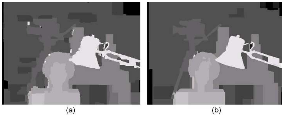
Fig. 13. (a) Standard belief propagation result. (b) Our enhanced global stereo method, given the knowledge of depth discontinuities.
