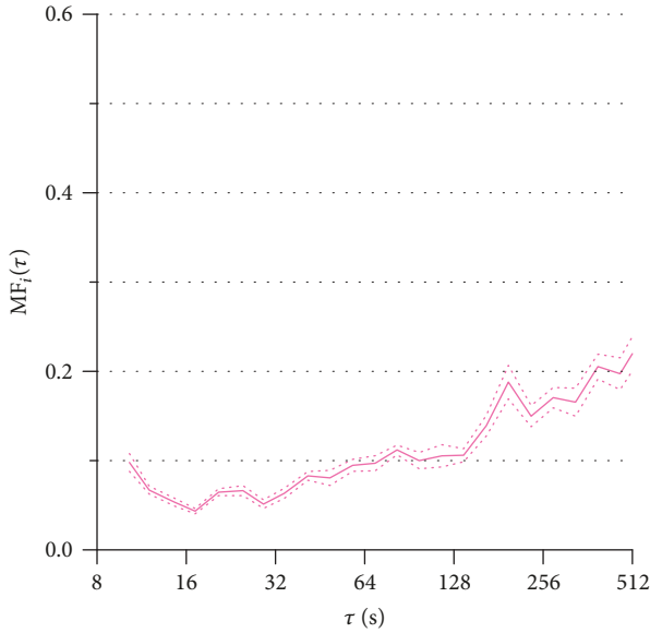
FIGURE 11: Multifractal index of pink noise. Median \pm standard error of the median for the 100 synthesized series of Figure 10.
