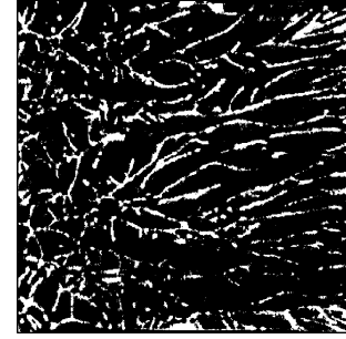
(c) PG membrane in 10 cm×10 cm tank, Ra = 2.03 \times 10^{11} , \Delta C = 3.198 g/l, Q = 0.11 mg/cm 2 /min, W_* = 0.31 cm/s, Re = 797 , Image area = 9.157 cm square, 728^2 pix
