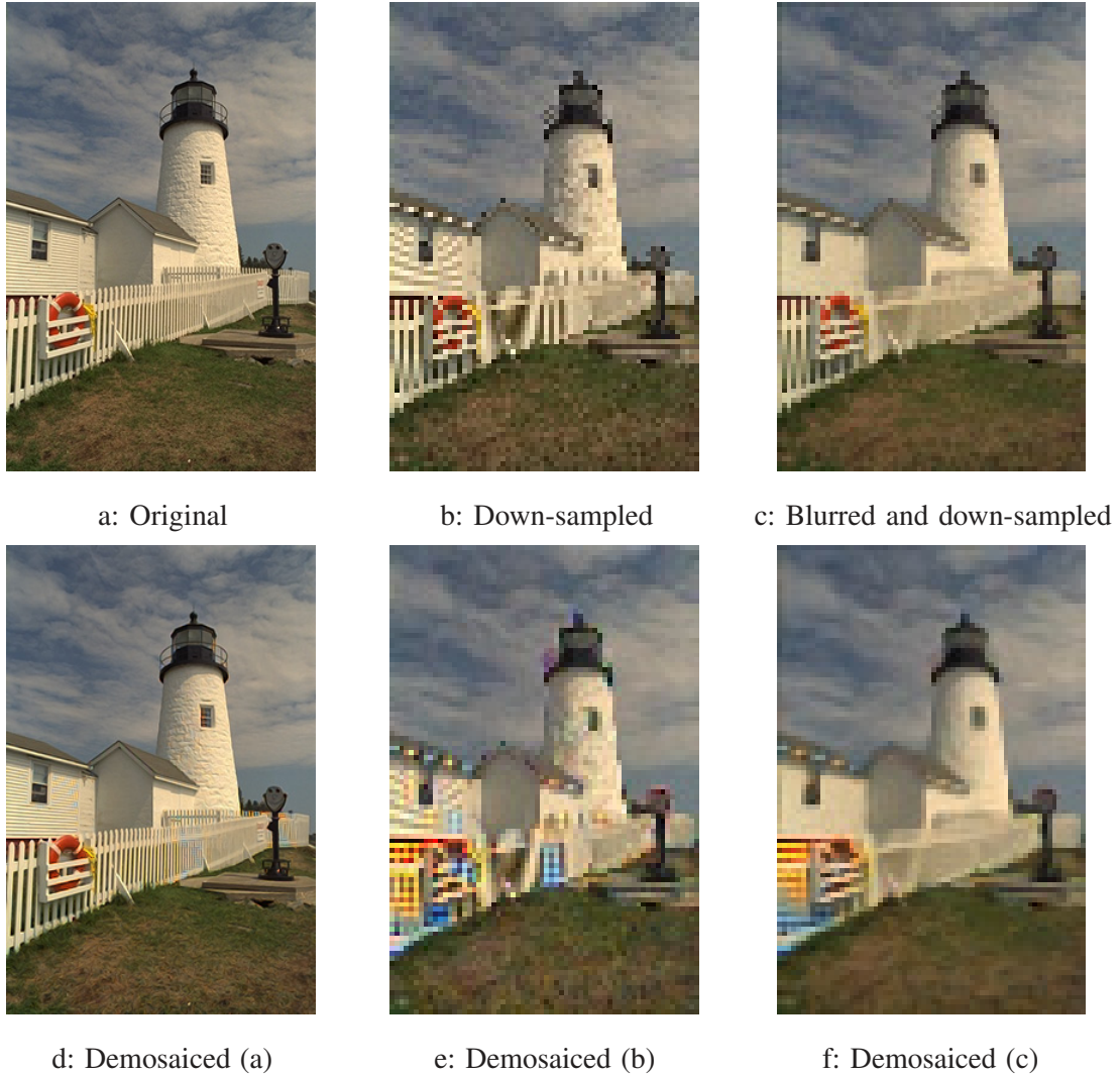
Fig. 2. A HR image (a) captured by a 3-CCD camera is down-sampled by a factor of four (b). In (c) the image in (a) is blurred by a Gaussian kernel before down-sampling by a factor of 4. The images in (a), (b), and (c) are color-filtered and then demosaiced by the method of [44]. The results are shown in (d), (e), (f), respectively.
