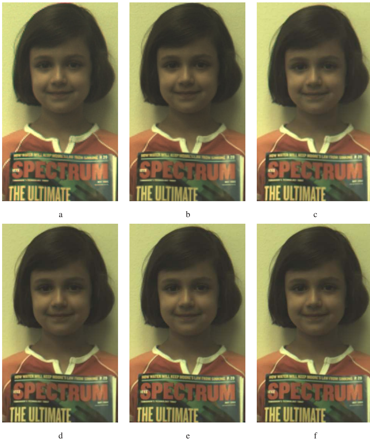
Fig. 11. Multi-frame color super-resolution implemented on a real data sequence. (a) shows one of the input LR images demosaiced by [14] and (b) is one of the input LR images demosaiced by the more sophisticated [44]. (c) is the result of applying the proposed color-super-resolution method on 31 LR images each demosaiced by [14] method. (d) is the result of applying the proposed color-super-resolution method on 31 LR images each demosaiced by [44] method. The result of applying our method on the original un-demosaiced raw LR images (without using the inter color dependence term) is shown in (e). (f) is the result of applying our method on the original un-demosaiced raw LR images.
