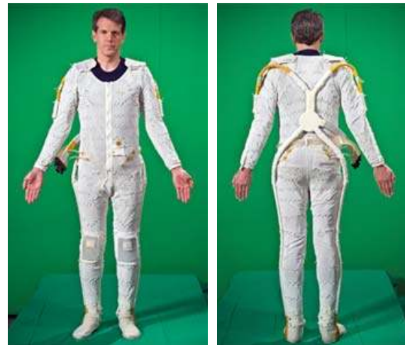
Figure 3. LCVG from the Extravehicular Mobility Unit (Jinny, does ILC have a better photo than this? –Mike) . 8
