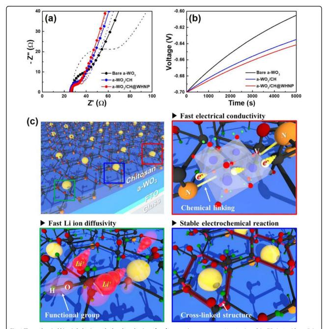
**Fig. 4 Electrochemical kinetic behavior and related mechanism of performance improvement. a** Nyquist plots of the EIS obtained from all the films before (circular solid line with circle) and after 1000 cycles (dotted line), **b** OCVD curves of the multifunctional devices assembled with gel polymer electrolyte and Pt films as the counter electrode, and **c** possible mechanism to improve electrochemical behavior due to chemical cross-linking between chitosan and WHNP.
