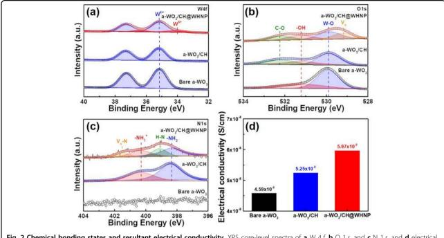
Fig. 2 Chemical bonding states and resultant electrical conductivity. XPS core-level spectra of **a** W 4 f, **b** O 1 s, and **c** N 1 s, and **d** electrical conductivity obtained from all the films.
