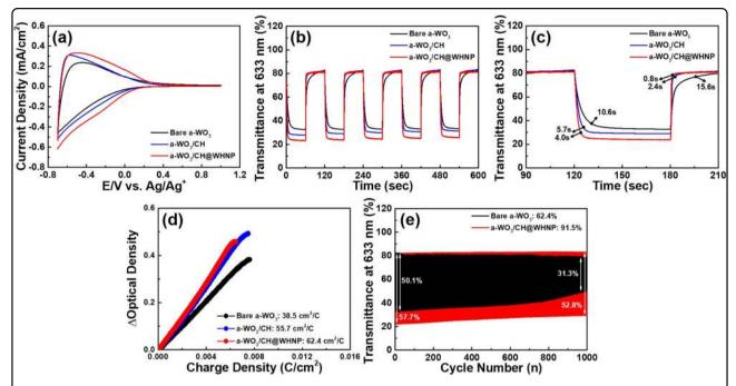
Fig. 5 Electrochemical and electrochromic performances. a CV curve of all films measured in the three electrode system in the potential region of -0.7 and 1.0 V (vs. Ag wire) at a scan rate of 20 mV/s,
