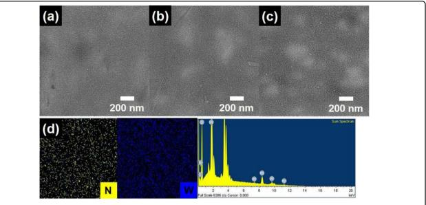
Fig. 3 Surface morphological characterization. a–c Top-view FESEM images of bare a-WO<sub>3</sub>, a-WO<sub>3</sub>/CH, and a-WO<sub>3</sub>/CH@WHNP, respectively, and d EDS result to show the existence of N and W elements of a-WO<sub>3</sub>/CH@WHNP.
