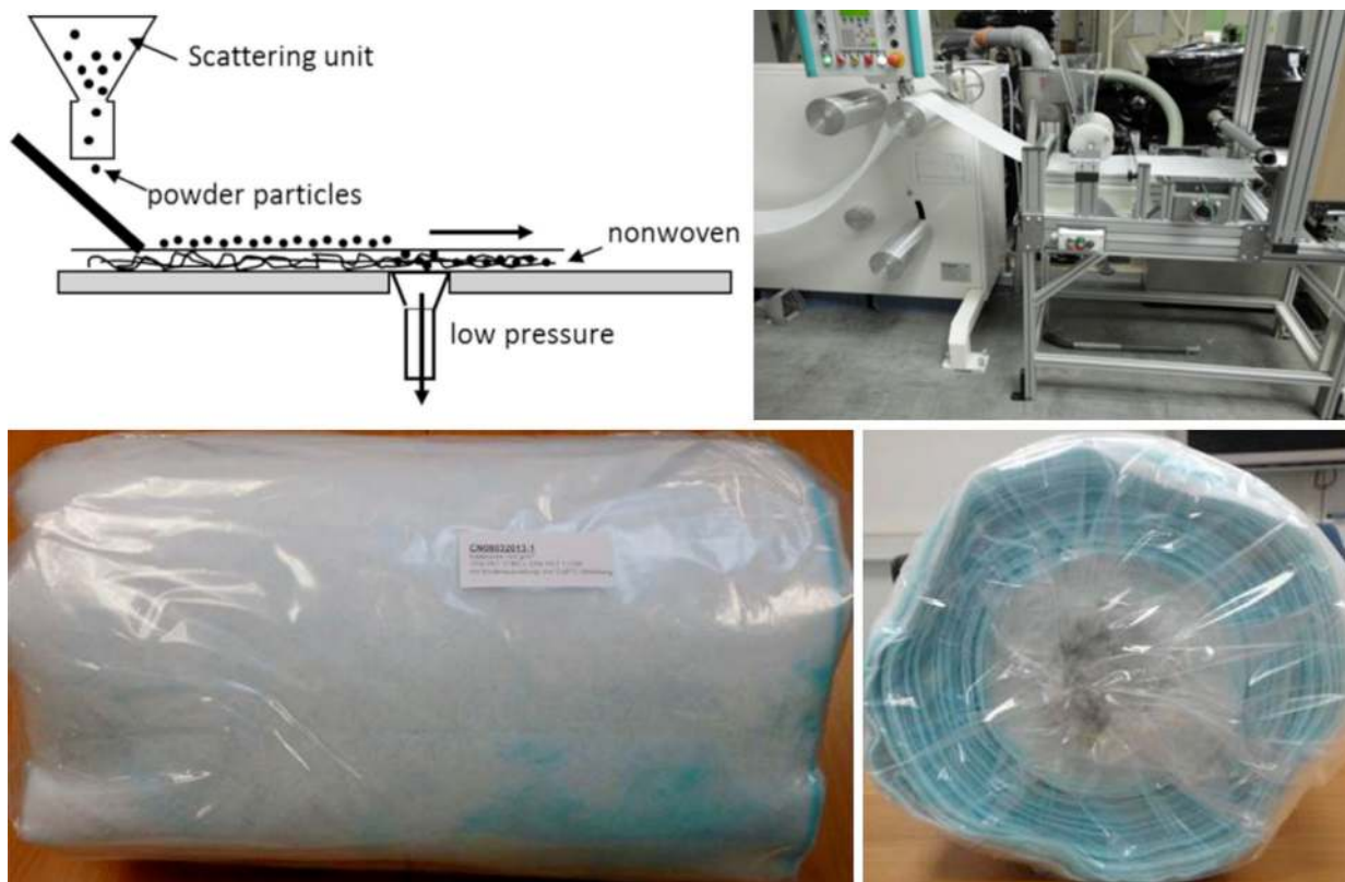
Figure 20 – Continuous and large-scale production process developed by Norafin in the context of NanoMOF project (reference FP7-NMP-2008-LARGE-2). ( Top left ) Principle of the dry loading process and ( top right ) the scattering-suction unit. ( Bottom ) Continuously MOF-particle loaded PET-nonwovens (HKUST-1 <math><63\ \mu\text{m}</math> from Johnson Matthey company; loading capacity: 25 g/m 2 ). [Reprinted from http://cordis.europa.eu/project/rcn/92877_en.html (accessed 02 March 2015).]
