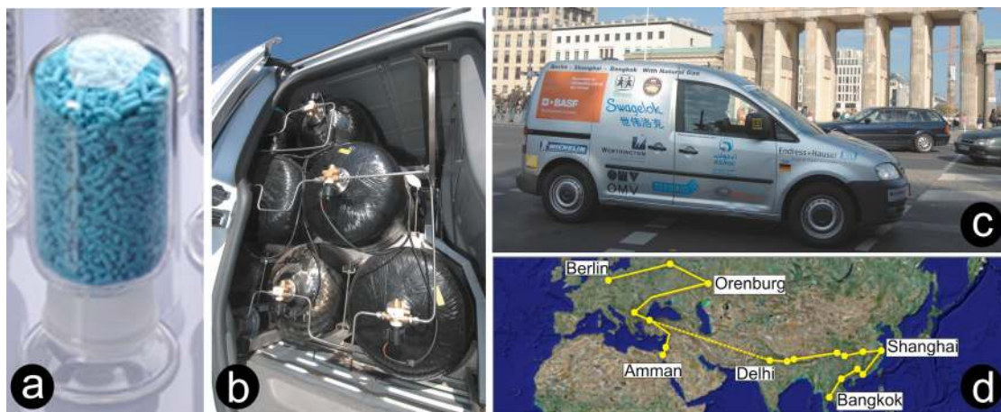
Figure 18 – EcoFuel Asia Tour 2007 - Berlin to Bangkok: 32 000 km with Basolite C300 in tank. (a) Basolite C300 (HKUST-1); (b) MOF-enhanced fuel tanks with CH 4 ; (c) Volkswagen Caddy EcoFuel prototype car; (d) journey map. (Adapted with permission from ref. 193.)
