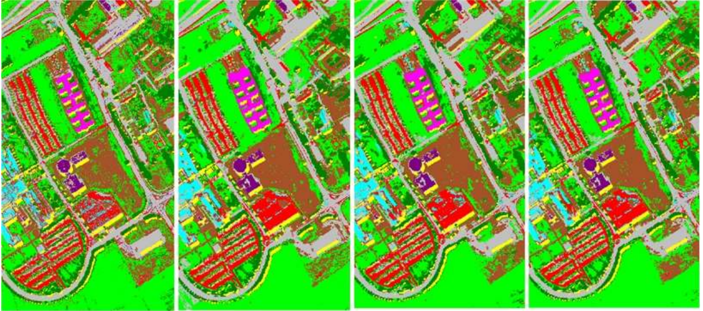
Fig. 11: The classification map of the standard SVM and the proposed classification method with 10-, 12- and 14-level segmentation by FODPSO
